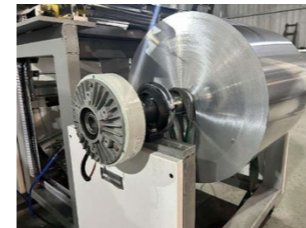
磁粉张力控制, 配自动过油 Magnetic powder tension control system with auto oiling
